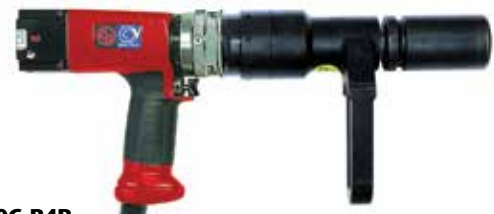
CPT7600C-R4P 1" BlueTork 4 Piston Nutrunner with Reverse • Short version with CUPS reaction bar in option • Selection up to 4 calibrated tightening torques • Air Shut-off clutch at preset torque
