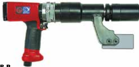
CPT7600XB-R 1" BlueTork Nutrunner with One Torque Preset and Reversible • Air Shut-off clutch at preset torque • Integrated reaction bar standard with blade
